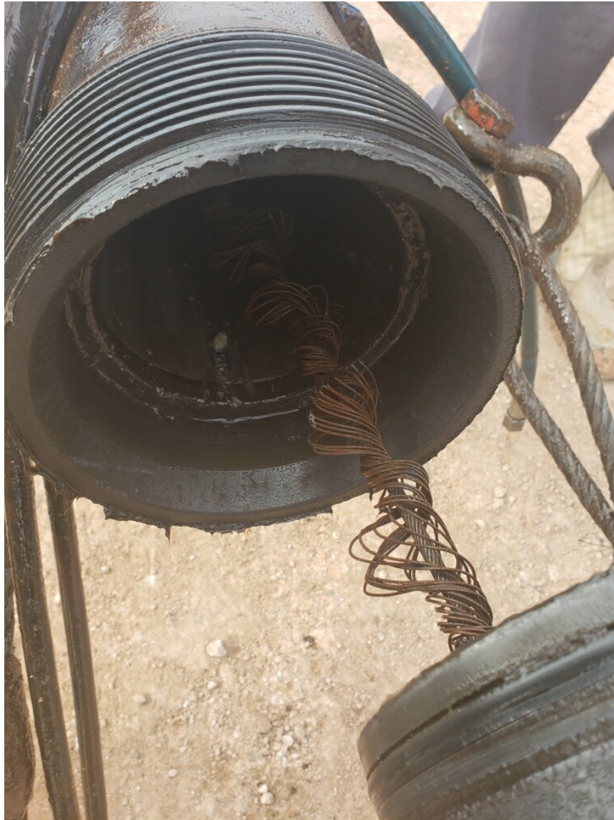
Birdcaged damaged Wireline
